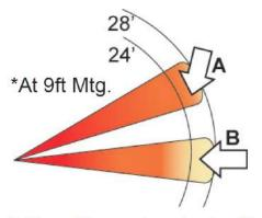
**A:** When walking across beam, detection will occur at approximately 28 feet. (8.53 m)
