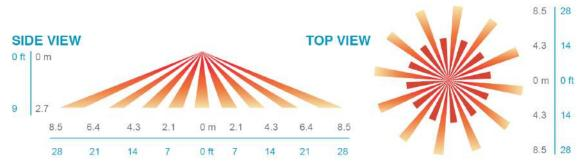
Sensors with Microphonics™ provides overlapping detection of human activity over the complete PIR coverage area. Advanced filtering is also utilized to prevent nonoccupant noises from keeping the lights on.
